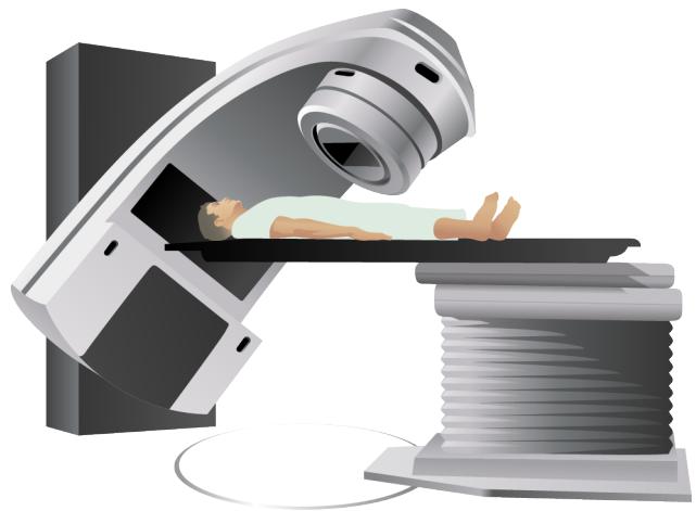
Figure 2.2: Radiotherapy machine with a rotating gantry, enabling treatment at different angles. Some treatment tables are able to rotate in order to enable more incidence angles.
