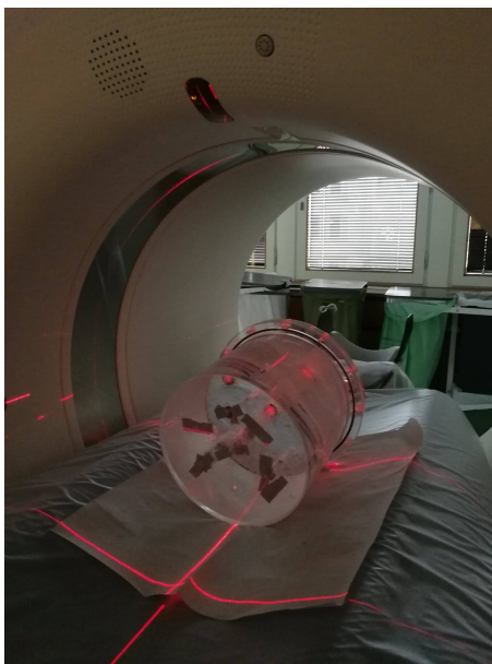
Figure 8: Phantom positioning at CT (left) and phantom with syringe inserts (right).
