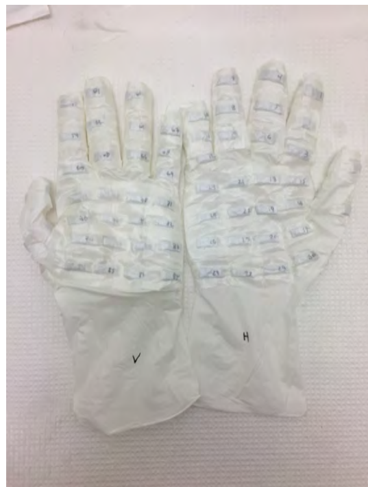
Figure 7. Examination gloves prepared with 3 NaCl pellets in each package. In total 54 measuring points for each glove.
