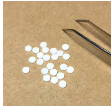
Figure 6. NaCl pellets used in the study, here compared with a standard tweezer.
