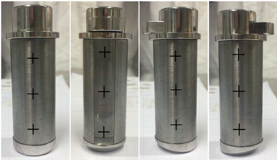
Figure 9. The positions of the measuring points (+) on the syringe wolfram shielding used when handling radiopharmaceuticals in syringes.
