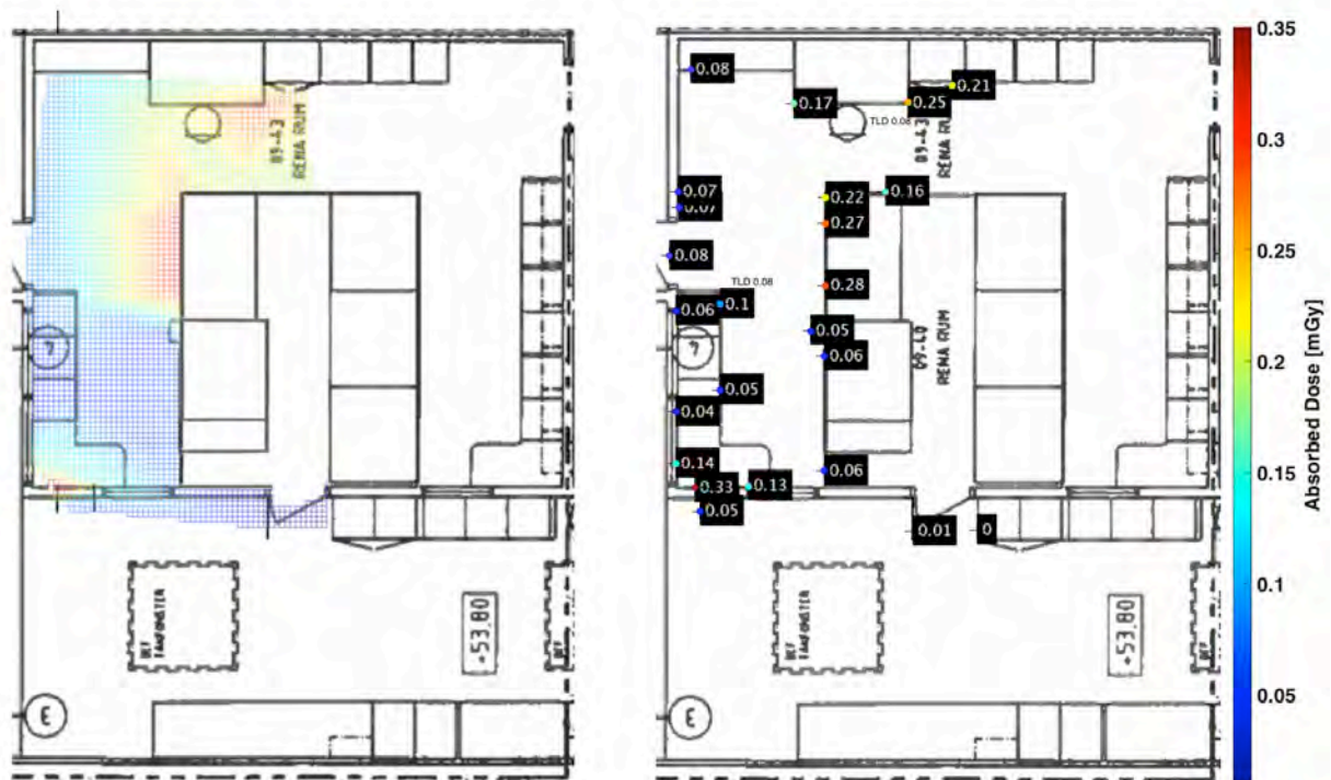
Figure 18. Left: Dose mapping, with interpolated values between measuring points, fused with the schematic drawing of the room. The errors of the absorbed dose for all measuring points are 7%. Right: Schematic view over the clean room and laboratory at the radiopharmaceutical preparation unit in Lund with the accumulated absorbed doses (7 days) marked at the position of the NaCl dosimeters. The reference TLDs both showed 0.08 mGy (from the picture is used with the kind permission of Birgitta Roos, SUS, Lund).
