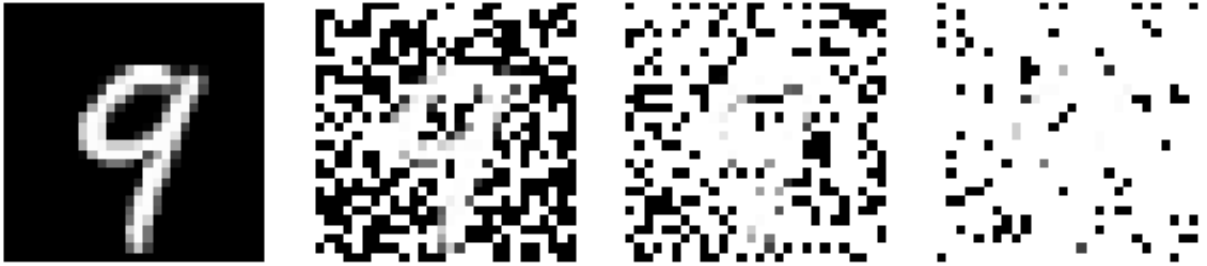
Figure 9: Example image with Random Pixels corruption. First: Original image. Second: 50 % corruption. Third : 70 % corruption. Fourth: 90 % corruption.
