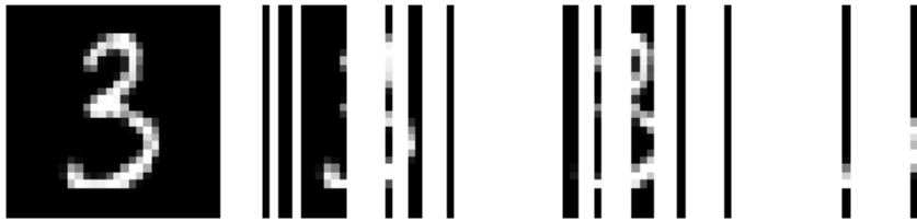
Figure 13: Example image with Vertical Lines corruption. First: Original image. Second: 50% corruption. Third : 70% corruption. Fourth: 90% corruption.
