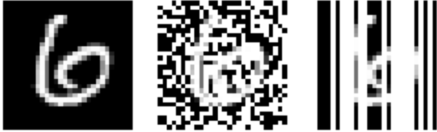
Figure 4: Left: original image, middle: Random Pixels 50% corruption; right: Vertical Lines 50% corruption.
