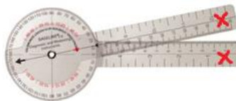
Figure 11: A goniometer. A BNO055 sensor was taped on each side (marked with red cross) to see if the calculated angle values were correct.
