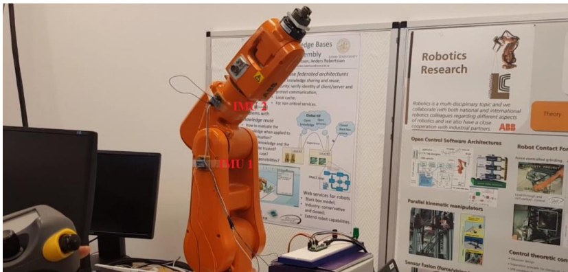
Figure 18: IMUs tested on a robot. Upper part of the robot arm was moving on different speeds, the results are presented in section 4.
