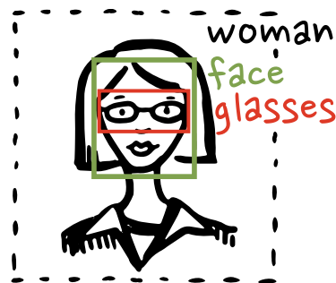
Figure 2.7: Annotating the input data may be done by placing coordinates around the parts of the image that are of importance.
