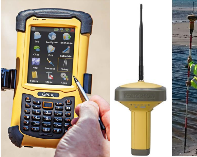
Figure 29. Topcon FC-336 mobile data controller(left), Topcon GR-3 receiver (middle) and the 2-meter long stick (right).
