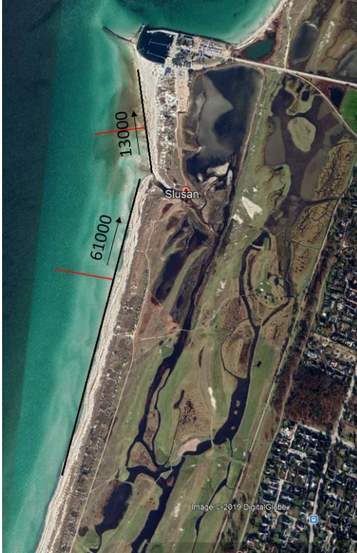
Figure 26. Net longshore sediment transport rate (in \text{m}^3/\text{year} ) along the west coast of Falsterbo.
