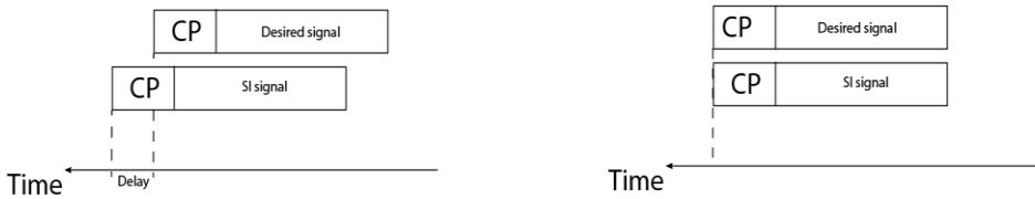
Fig. 2.10. Synchronization via time alignment.
