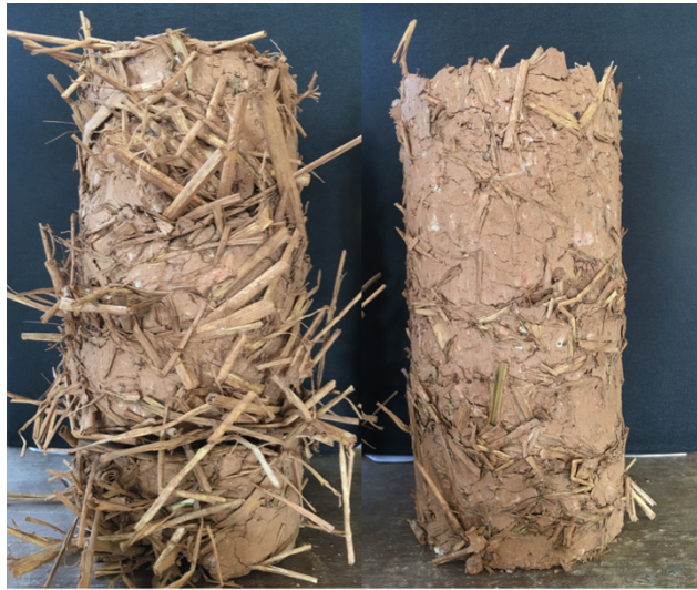
Figure 15: Two samples with 2 % straw by weight, 100 mm fibres(left), 20 mm fibres (right)
