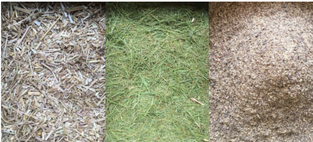
Figure 14: Used fibres, from left to right: straw, pine and raw rice husk
