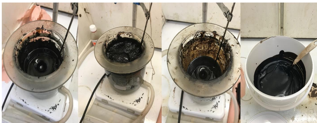
Figure 13. The pictures from left to right shows the proceedings of the sample homogenization. Left: Lignin has been dissolved into acetone/water/surfactant mixture. Middle left: Mixture of lignin/acetone/water/surfactant/VGO at boiling point around 52-92 °C Middle right: Mixture of lignin/surfactant/VGO round 92 °C Right: Lignin/surfactant/VGO mixture mixed with a larger bulk of VGO, about 10 w% lignin.
