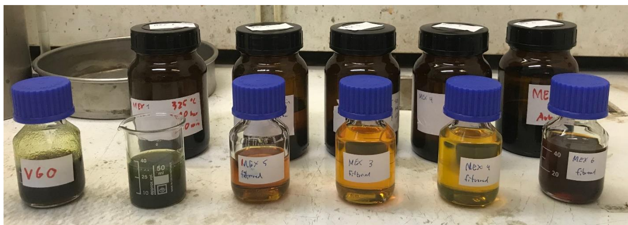
Figure 14. From left to right: Untreated VGO, MEX 1, MEX 5, MEX 3, MEX 4, MEX 6. The ordering of MEX 5, 3 and 4 is by increased time.
