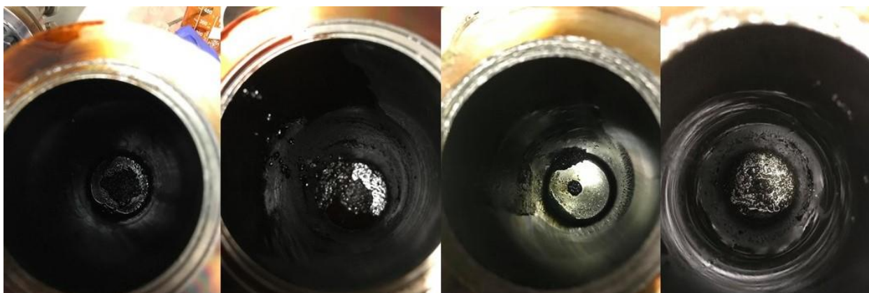
Figure 22. Picture showing coke found in the reactor after the following experiments from left to right: MEX13, MEX13.1, MEX 14 and MEX14.1 The pictures shows that a lot more coke was found in the lignin experiments upon opening of the reactor.
