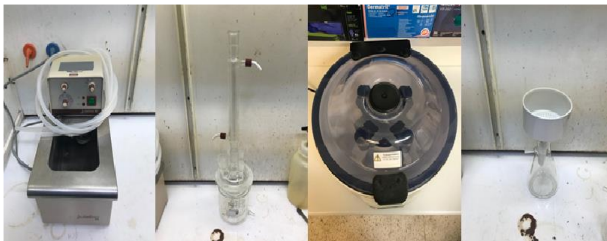
Figure 8. Equipment used for POLO from left to right. 1: Water bath. 2: Mantled glass reactor with the bottom part being connected to 1 for heating and the top part being used for cooling of fumes. 3: Centrifuge. 4: Vacuum filter flask with Buchner funnel on top.
