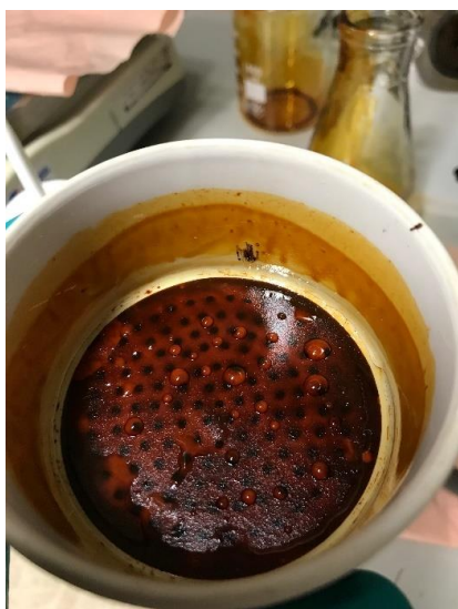
Figure 18. Assumed water droplets found after filtrating the liquid content in the reactor following experiment containing lignin mixture.
