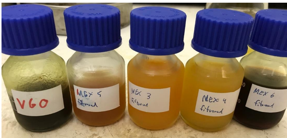
Figure 15. From left to right. V60, MEX 5, MEX 3, MEX 6 and MEX 6. The samples have just been taken out from the fridge and all except for MEX 6 shows semi-solid behaviour.
