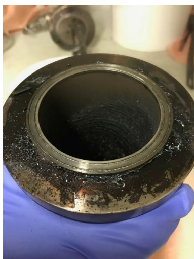
Figure 29. Burnt material found outside of the reactor following an experiment.
