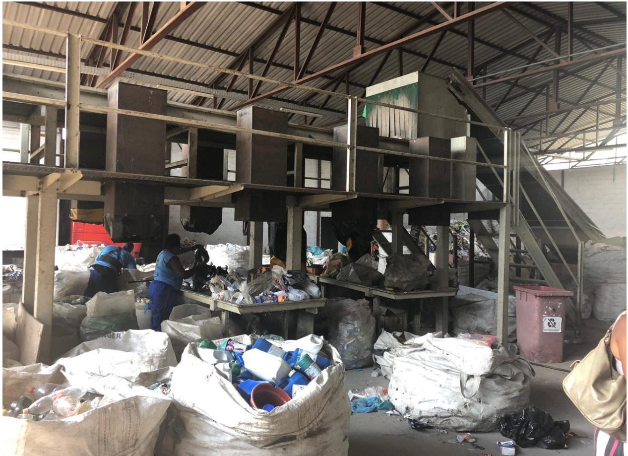
Figure 17 Separation process of another cooperative in Jardim Gramacho. They used to have rolling bands which would drop the waste on to the tables but since it broke the workers lift the waste bags onto the tables to sort. Photo: Emma Bergman 20/5/2019.
