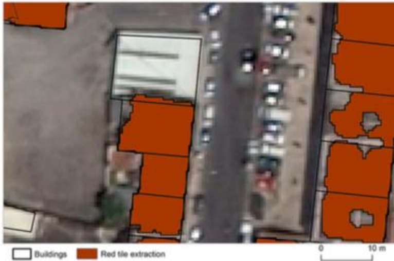
Figure 7: A picture of red-tiled roof classification done with a GIS tool (Santos et al. 2016).
