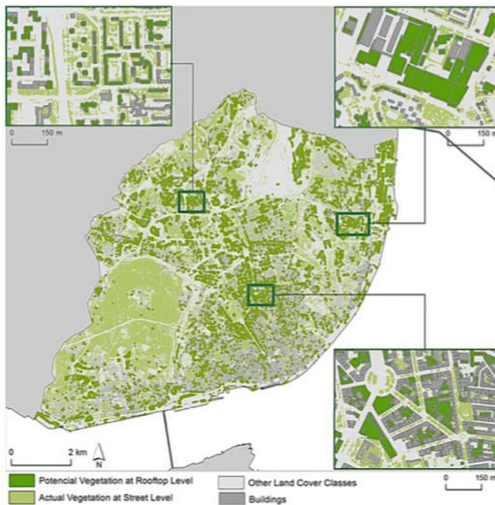
Figure 8: The dark green colour represents the potential green roof cover that can be built considering the flat and pitched green roof and shaded to sunny scenario (Santos et al. 2016).
