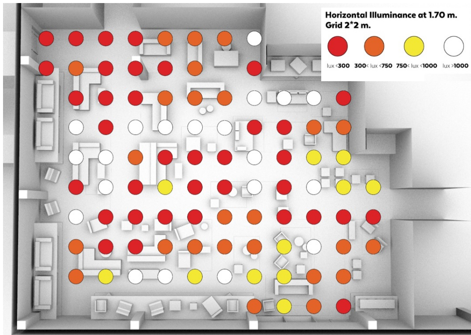
Figure 37: Horizontal illuminance average measurements during night-time at Living Room department.
