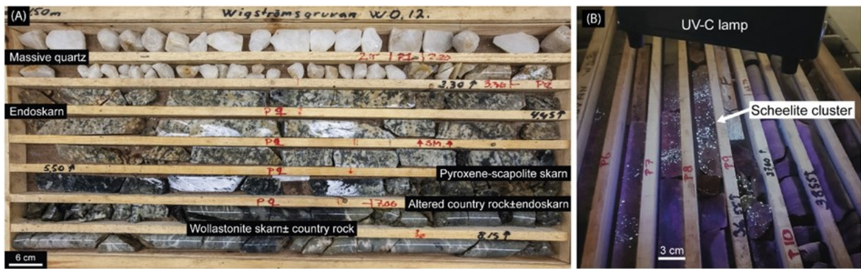
Fig. 5. 5a: Example of a drill-core box at Malå, Sweden. 5b: Scheelite "glow" under UV-C light.
