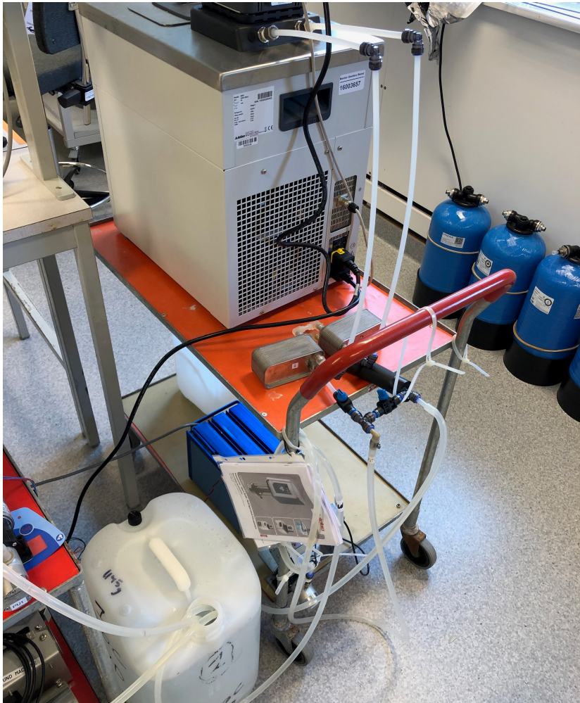
Figure 4.8 Water circulator and water tank
