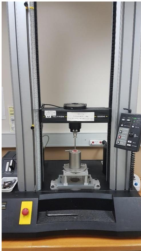
Figure 19 The Instron with a loaded syringe.
