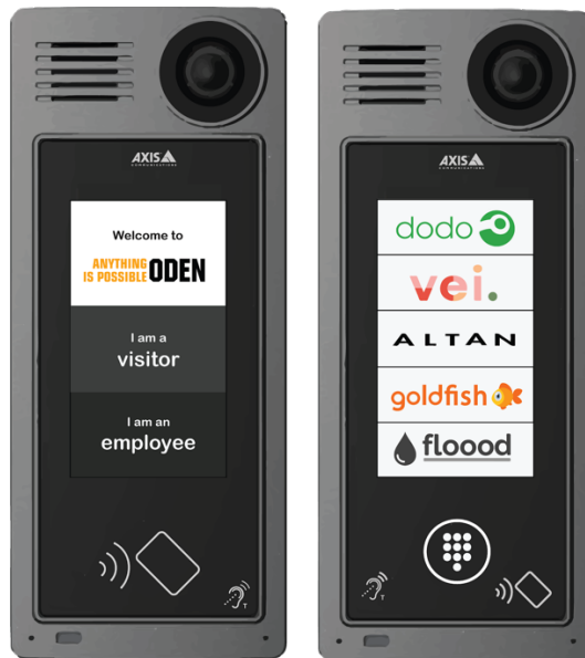
Figure 8.4 The design of the whole solutions with the start pages of the final concepts. The Display only concept is on the left and The Button concept is on the right.
