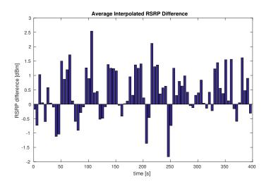
Figure 7.10: Difference between interpolated values in machine learning and baseline over all measured RSRP values in road mover scenario.
