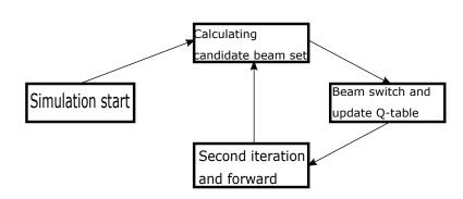
**Figure 5.1:** Block-scheme showing the structure of the implemented machine learning algorithm.
