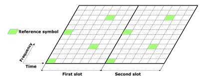
Figure 3.4: Structure of CRS within a resource block pair.
