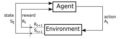
Figure 4.1: Block-scheme over Reinforcement learning process.
