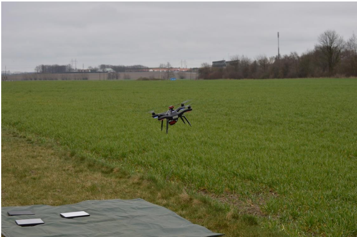
Figure 9: Reflectance panels setup during actual UAV data collection mission at Lönnstorp..Photo: by Ashish Vivekar.
