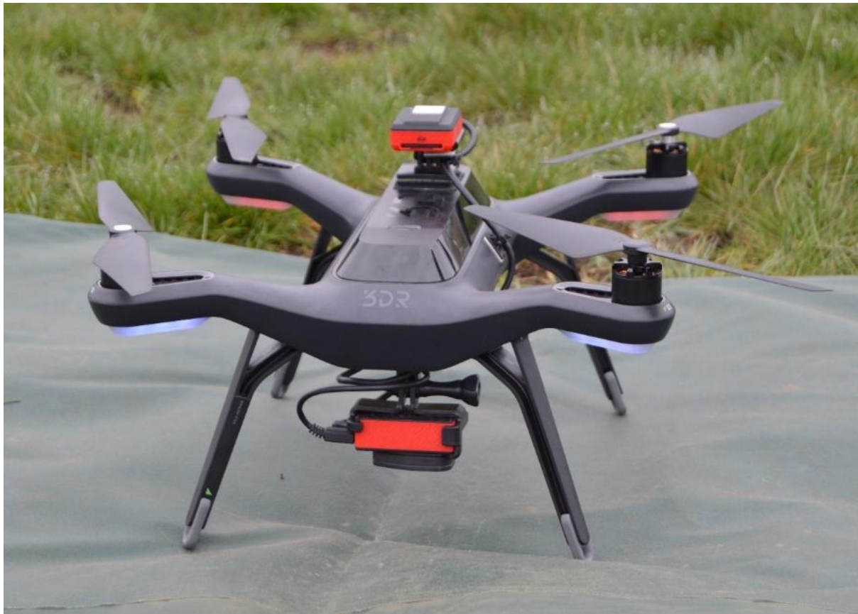
Figure 6: 3DR Solo UAV mounted with Parrot sequoia multispectral sensor and sunshine sensor. Photo: by Ashish Vivekar.
