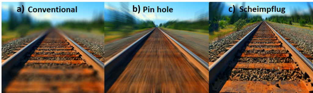
Figure 1.3: Comparison between conventional, pin hole and Scheimpflug photography on images taken from a train. Image credit Malmquist et al. [8].
