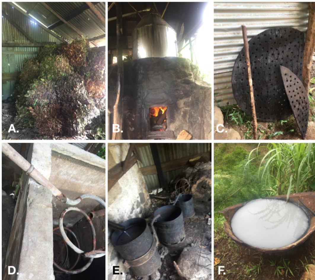
Figure 11: photos of artisanal distilleries from field visits. A: harvested leaves being dried for distilling, this is approximately the amount of leaves for one batch. B: A fire heating the vat on top of it. C: A damaged tammy. D: A common but old-fashioned design of a condenser, when the process is running it is covered with flowing water: E: One of the separation methods. F: waste water container with heavy oil in the bottom.
