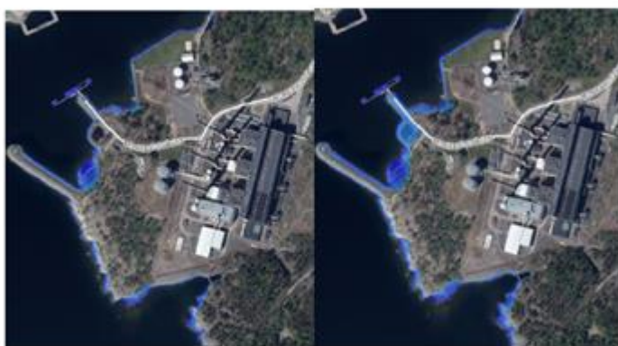
Figure 35: Power plant area in SCALGO Live. Left: Design sea level today (155 cm); right: Design sea level in the year 2100 (240 cm).
