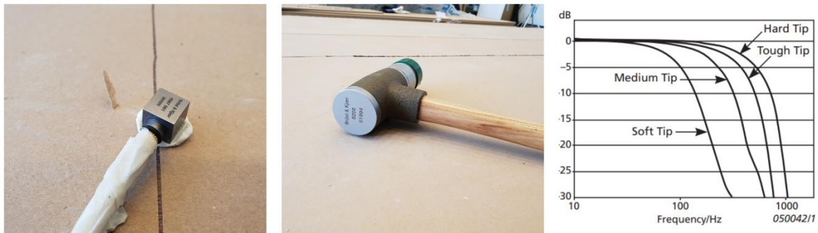
Figure 13. Bruel & Kjaer accelerometer (left), Bruel & Kjaer modal hammer (middle), hammer tip diagram (right)
