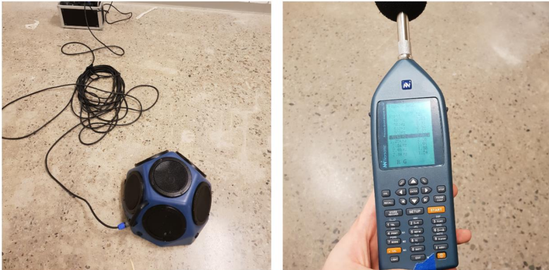
Figure 23. Measurement equipment. Loudspeaker (left) and sonometer (right).
