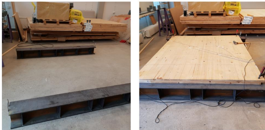
Figure 56. Measurement setup, 3-layer CLT
