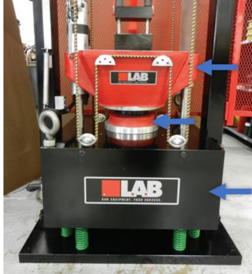
Figure 4.2, The carriage, the programmer and the impact block of the SD-10 shock-testing machine from L.A.B. Equipment [9].
