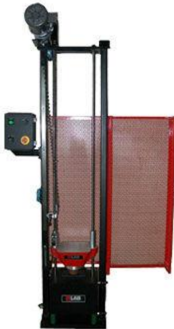
Figure 4.1, The SD-10 shock-testing machine from L.A.B. Equipment [9].
