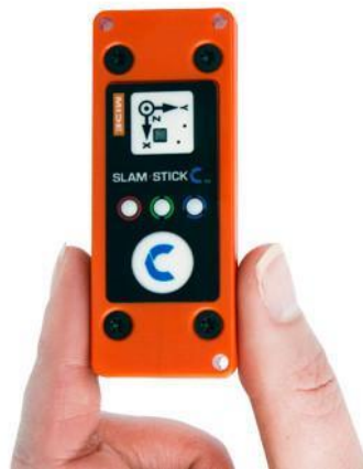
Figure 5.1, The Slam Stick C from Mide Technology [12].
