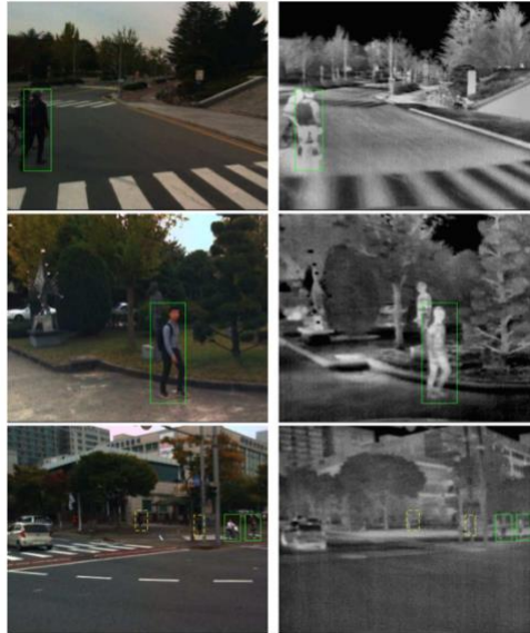
Figure 10 Regular monocular imagery and multispectral images shows detected pedestrians. Image from (Guan et al., 2018)
