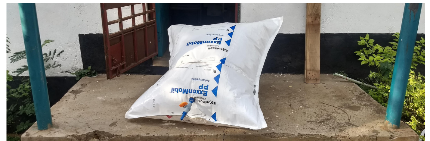
FOUR DIFFERENT BAGS SPLICED TOGETHER. WITH THE CONNECTION TECHNIQUES AT OUR DISPOSAL, GUARANTEING AIR-TIGHTNESS PROVED EXTREMELY DIFFICULT.
