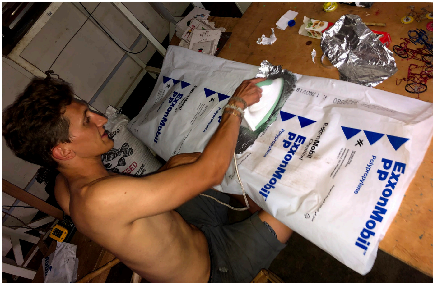
PROTOTYPING A LARGE BAG BY MELTING THE PLASTIC AIRTIGHT WITH AN IRON
