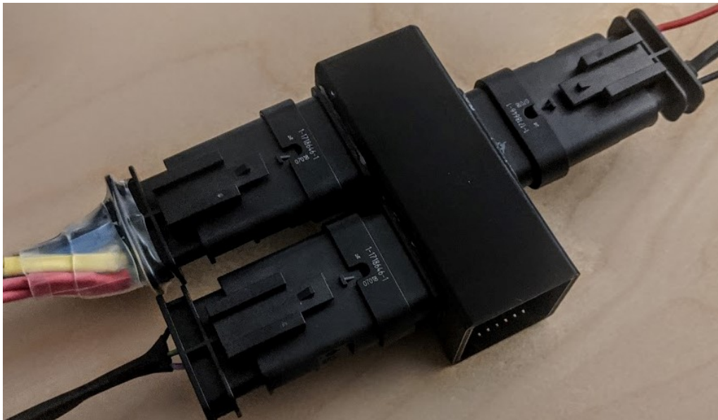
Figure 5.11: The final assembled TVECU, with connections to FS CAN, TVDC CAN and simulated TVDC sensors.
