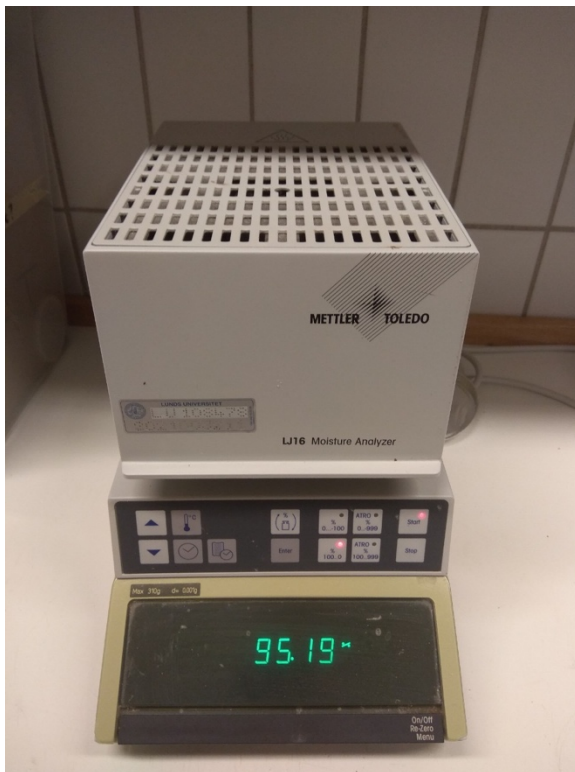
Picture 5 . Moisture analyzer (used for all moisture analysis in this experiment).
