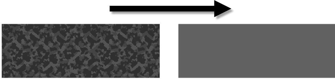
Figure 2: Schematic illustration of a solid solution treatment process. Cast specimen with solid precipitates (left) is heated until composition is homogeneous (right).
