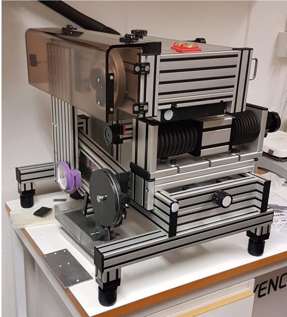
Figure 8: Automatic diamond wire saw used for cutting specimens, with oil lubricant.
