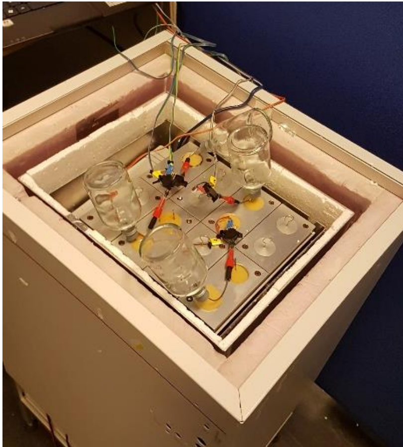
Figure 9: Loaded calorimeter with pressure sensors connected.
