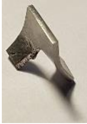
Figure 10: Cut and flared specimen for pH test.
