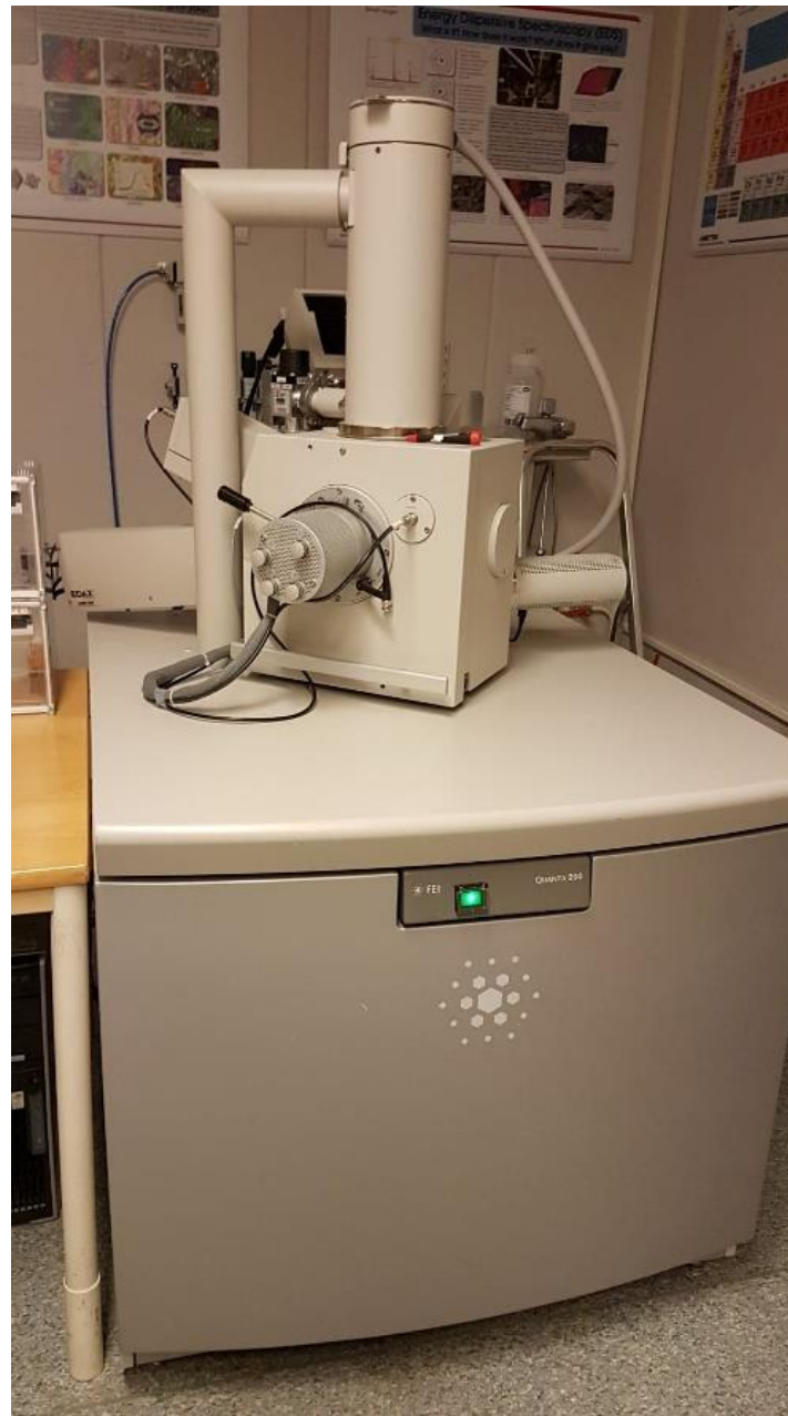
Figure 11: FEI Quanta 200 Scanning electron microscope (SEM).
