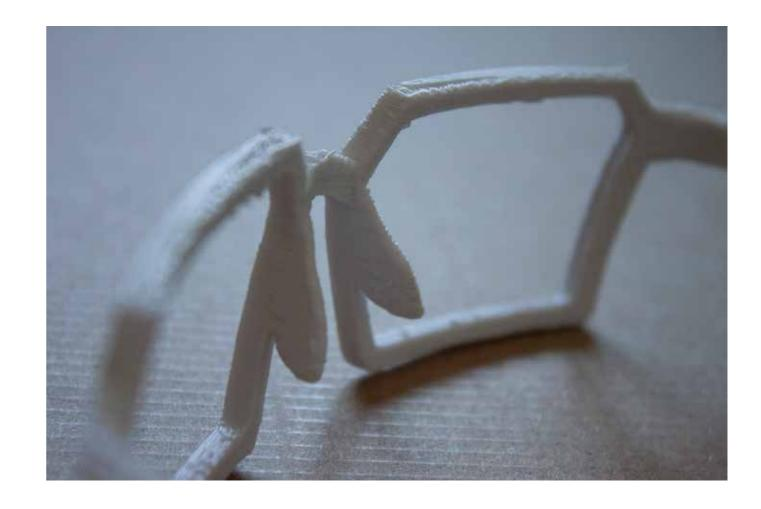
3D printing has been the main tool for prototyping in my project. I worked in fusion where I used two of the laser cutting models. I did a lot of different measurements, different width, height, bending, etc. I also realized even more how great the 3D prints worked as a final material. It is very lightweight and can be made into a personalized final model for every face shape.
