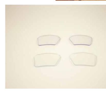
I wanted to add lenses to my frame to make the prototype complete and even more professional. At first, I tried to make them on my own in plexiglass with a heating gun. This created bubbles because of the heat and the edges were not as precise as I needed them to be for the trace in the frame. I went to an optician with my 3D printed frame and got good quality lenses that would fit my frame perfectly.
