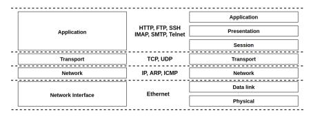
Figure 2.1: The TCP/IP model compared with the OSI model.
