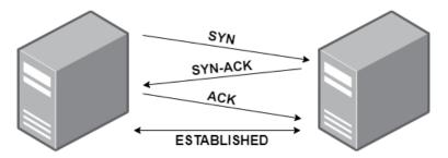
**Figure 2.4:** TCP connection establishes through a three-way hand-shake.
