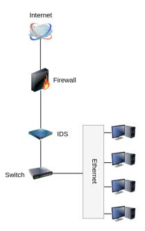
Figure 2.10: IDS placement inside a network.
