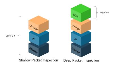
**Figure 2.12:** Visual comparison of inspection range between shallow and deep packet inspection.
