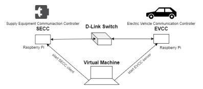
**Figure 3.1:** Hardware setup for the project development environment.
