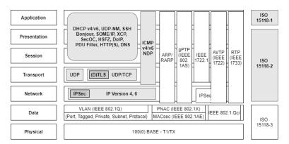
**Figure 2.7:** An ISO model of ESCRYPT's CycurGATE. Protocols used for vehicle communication, with protocols in grey representing protocols used over automotive Ethernet [35].
