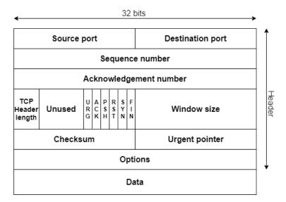
Figure 2.3: TCP header
