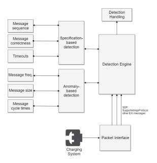
Figure 5.1: Illustration of the implemented IDS.
