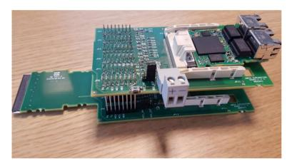
Figure 5.5: Anybus CompactCom traffic interceptor.
