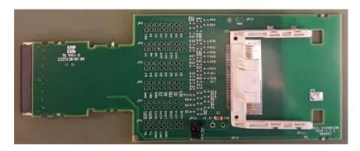
Figure 5.2: Anybus CompactCom Expansion Board 023070-B.
