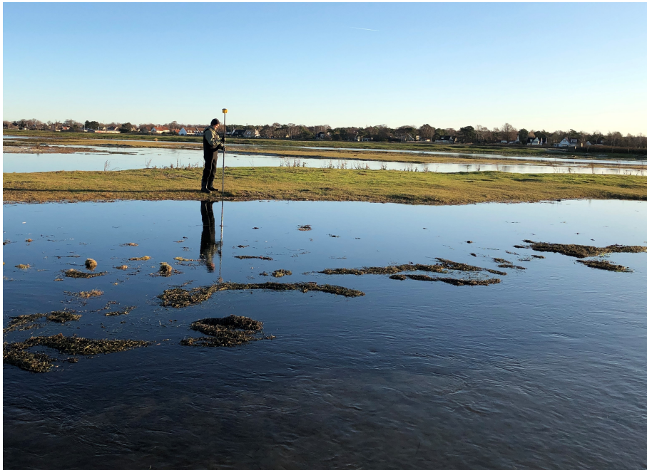
Figure 25: Bathymetry measurements carried out in Flommen by using a SPS985 GNSS Smart Antenna. Photo by: Clemens Klante
