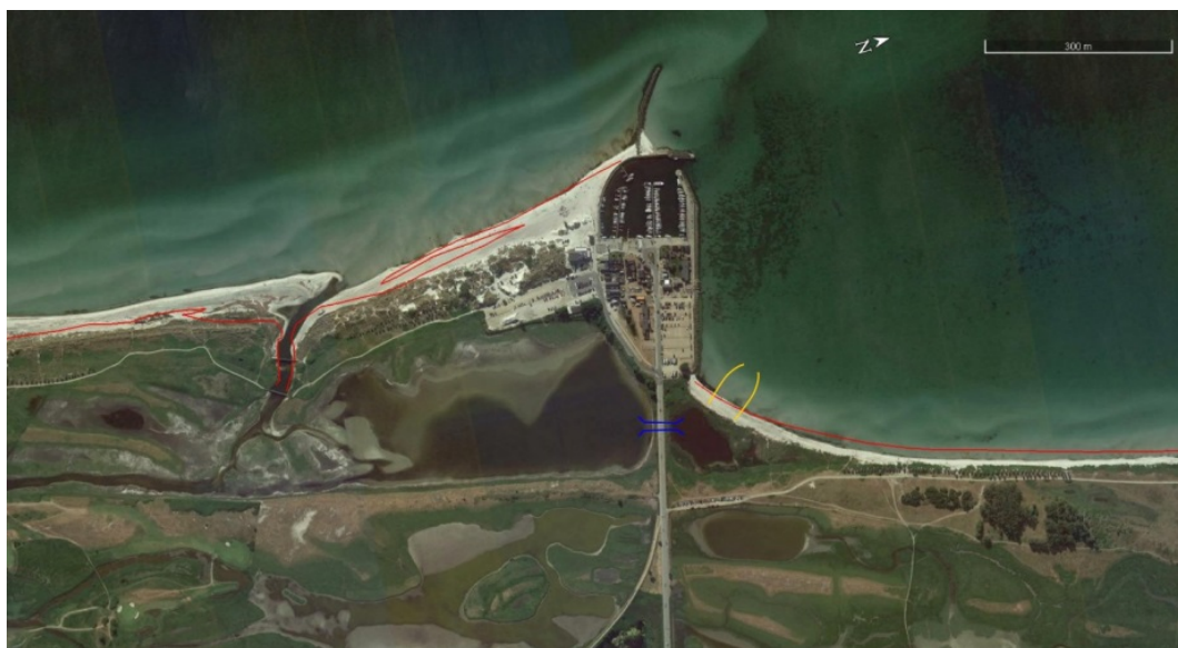
Figure 45: Suggested inlet north of the harbour. Yellow lines signify the proposed jetties. Blue lines under the Skanör Harbour Road signifies the new canal. The red lines indicate the 2007 coastline (Danish Hydrological Institute, 2018).
