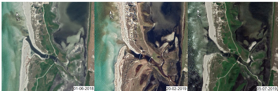
Figure 15: Picture of the inlet Slusan in Flommen Lagoon showing the varying geometry and location of the inlet (Maxar Technologies, 2019).
