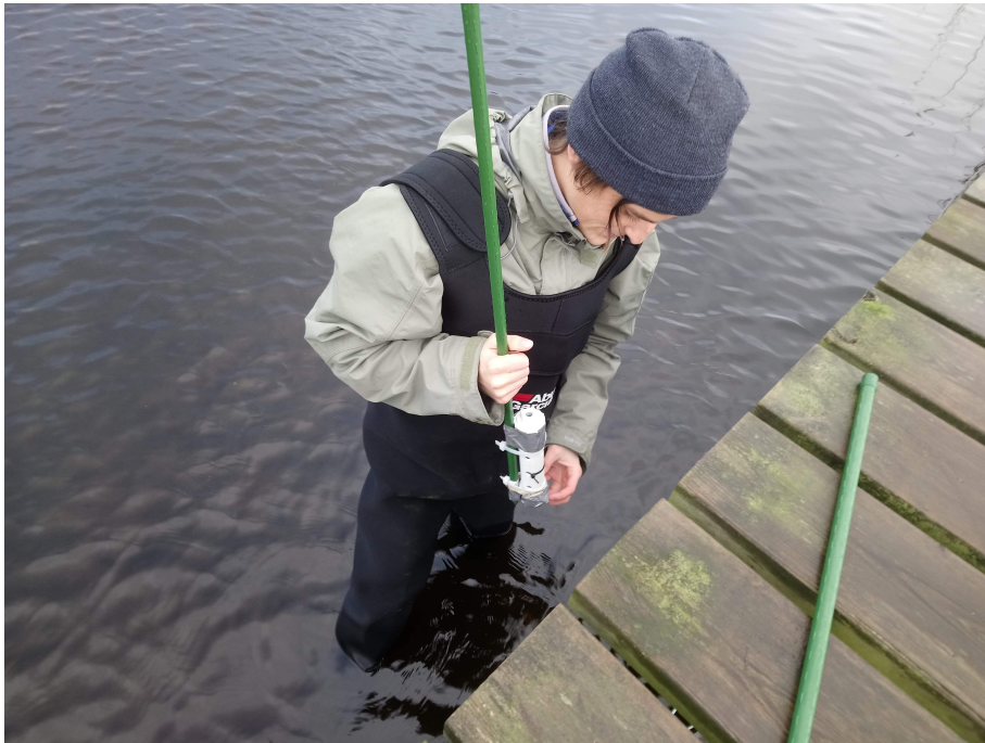
Figure 23: A picture showing the deployment of a water logger. The water logger is deployed by attaching it to a bridge pier. Photo by: Kenny Lay
