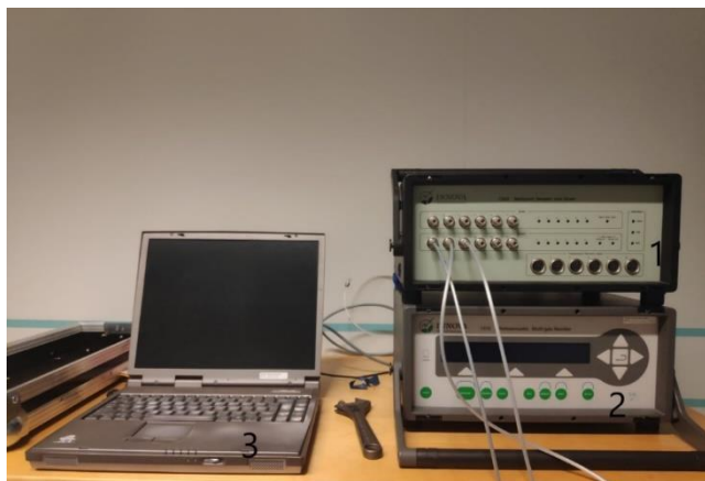
Figure 18 1. Air sampler, 2. Analyzer, 3. PC with innova software. Tracer gas setup
