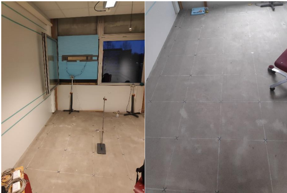
Figure 15 Swema draft equipment and the space with measurement points marked on the floor
