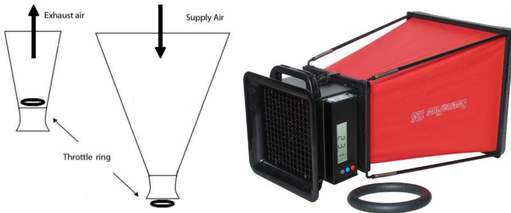
Figure 13 (a):Ring placement, (b):actual equipment
