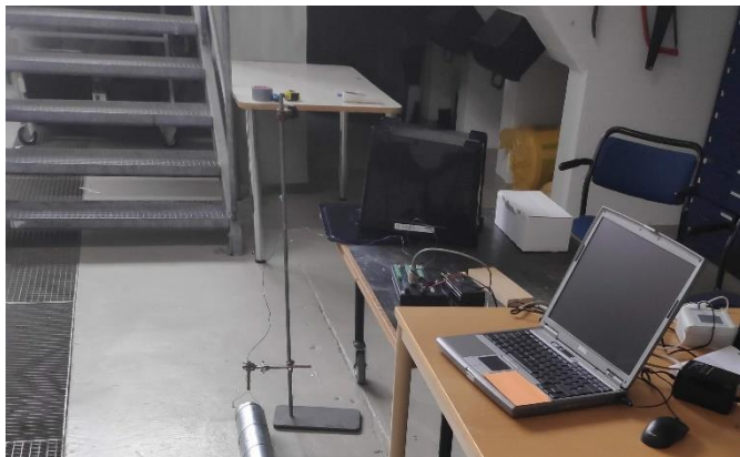
Figure 10 Thermocouple test station, Box and Duct
