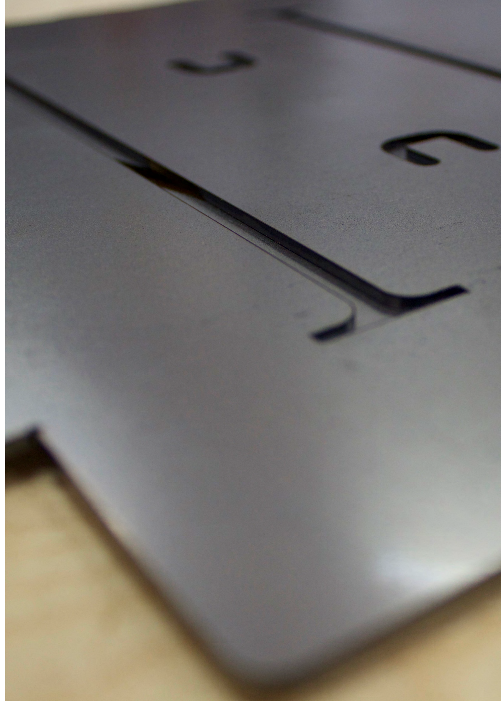
Fig. 60: Lasered sheet metal feet
