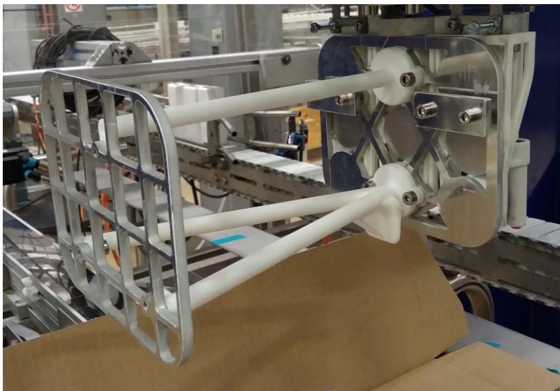
Figure 41: Push attachment attached to gripper head
