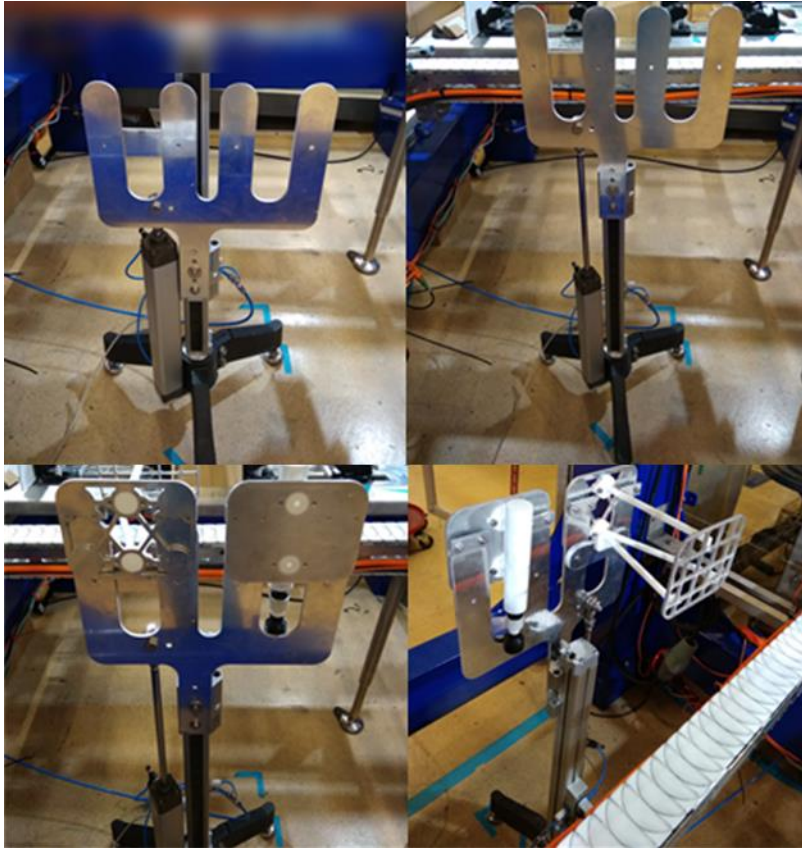
Figure 26: Holder retracted (upper left) & extended (upper right), with attachments back (lower left) & front (lower right)
