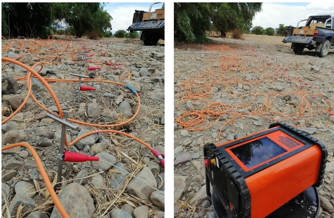
Figure 6. Pictures of the cable and steel electrodes (left) and ABM Terrameter LS 2 resistivity meter (right) used in the field work.
