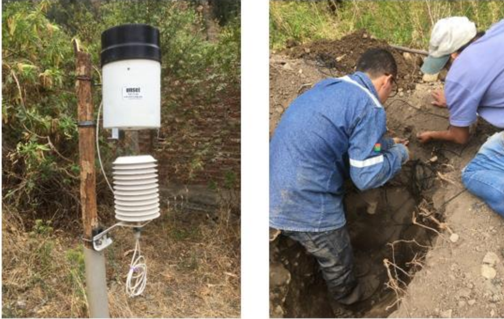
Figure 7. The assembled Onset rain gauge (left) and the installation process for the soil moisture sensors (right).
