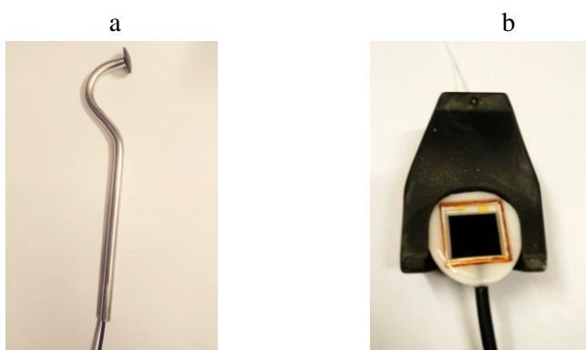
Fig. 9 Fiber probes. Figure 9a contains the probe that was used for measurements inside the mouth. Figure 9b, instead, contains the probe that was used for measurements outside the mouth. This probe contains the fiber on the top part and the detector on the bottom part. See figure 11 to better understand how the two probes were used for the measurements.
