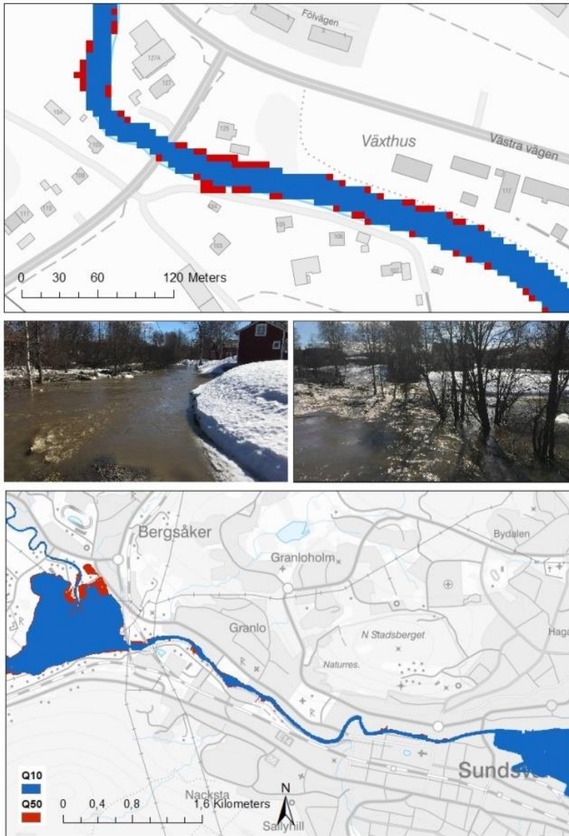
Figure 14. Photographs from the event the 21-23 rd of April in 2018 compared with corresponding simulated flow event with return times 10 and 50 years 83 . Approximate coordinates for the location of the images: [E614692, N6922062] (in meters)
