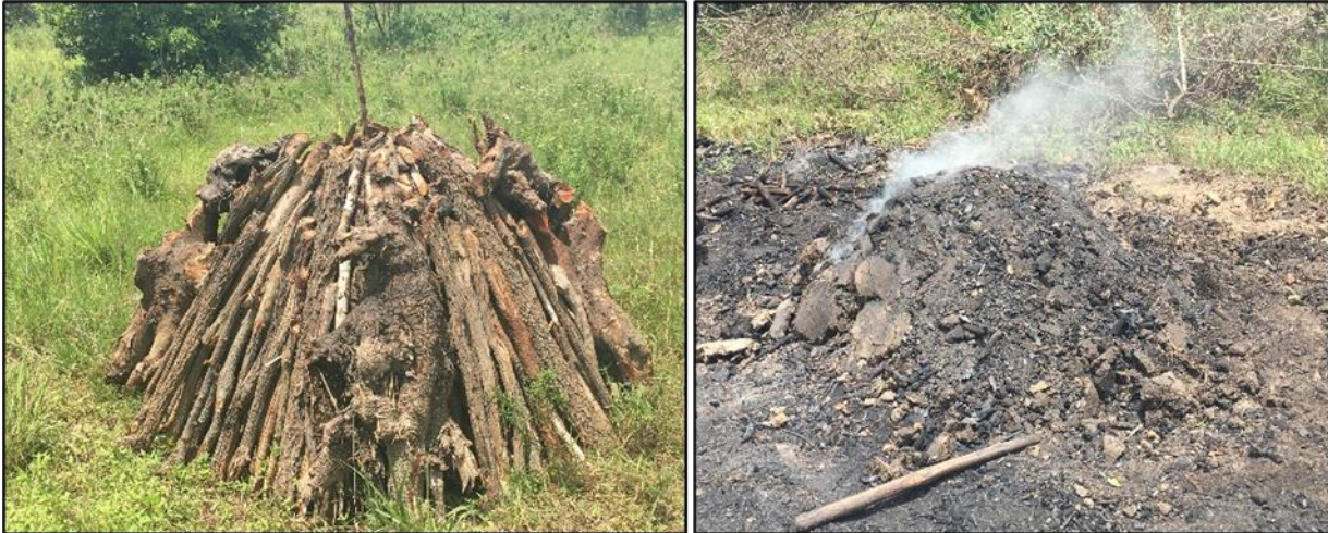
Figure 7. Traditional earth kilns in Kisarawe. To the left: kiln prior to burning. To the right kiln whilst burning (Photo by author Jan. 28, 2020, Kisarawe).
