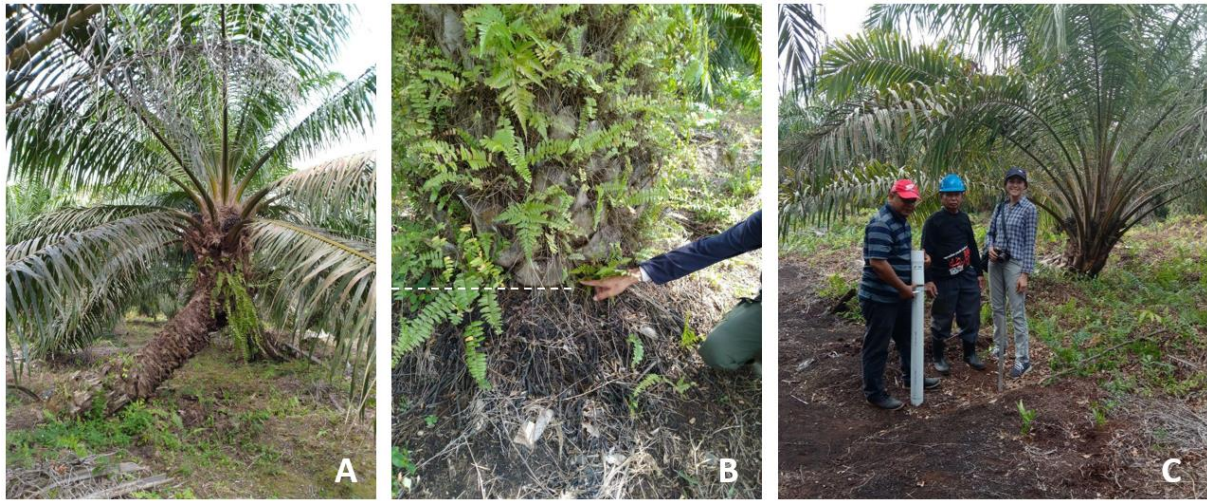
Figure 19 The consequences of peat subsidence: a) collapsed oil palm tree, b) the soil level when the tree was first planted, c) a measurement pipe for soil moisture monitoring. (Photos by the author and a smallholder in Siak, January 26, 2020)
