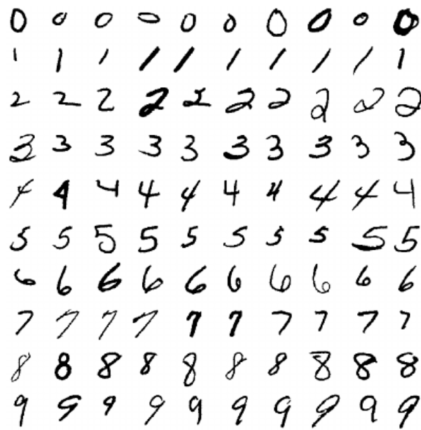
Figure 3.1: Raw data from the MNIST database, from C.-L. Liu et al. 2003. Each of the shown digits corresponds to a 28x28 pixels bitmap (image) containing grayscale values.
