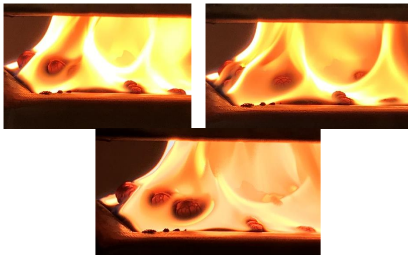
Figure 29 Composite sample burning
