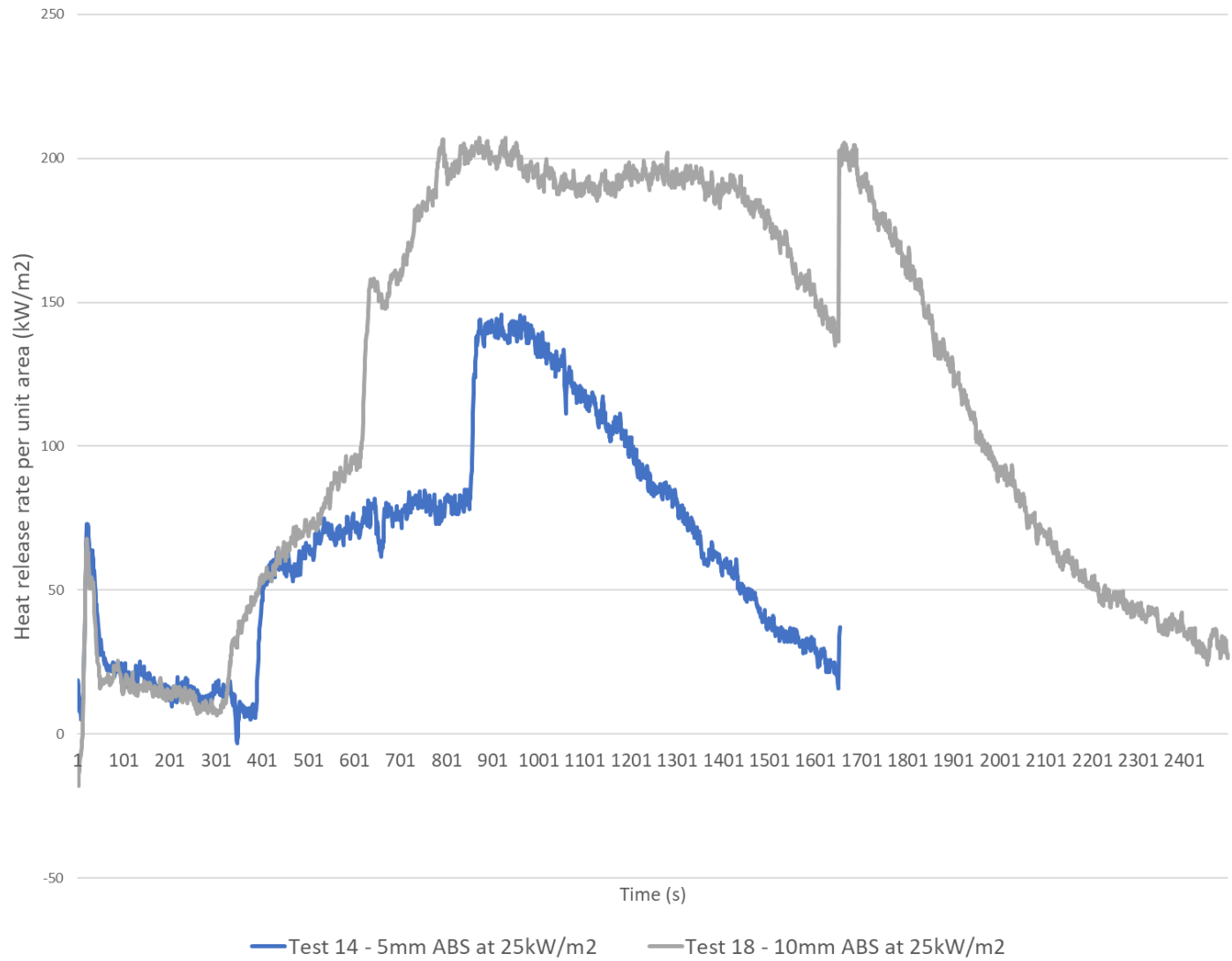
Average heat release rate per unit area ( \text{kW/m}^2 ) values for composite samples at 15% \text{O}_2
