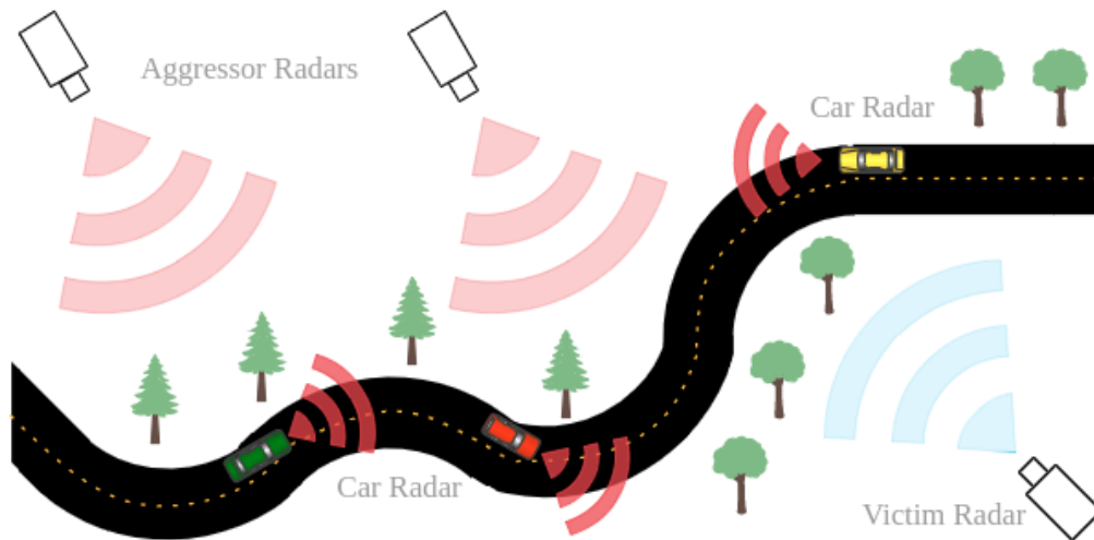
Figure 2.14: Schematic representation of interference from other radars.
