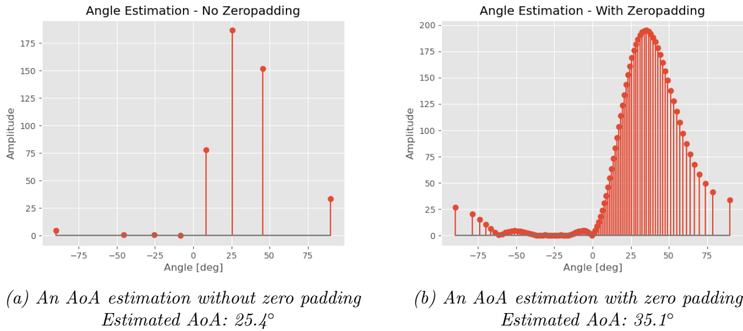
Figure 2.4: AoA estimation with and without zero padding - Object AoA: 35.0°
