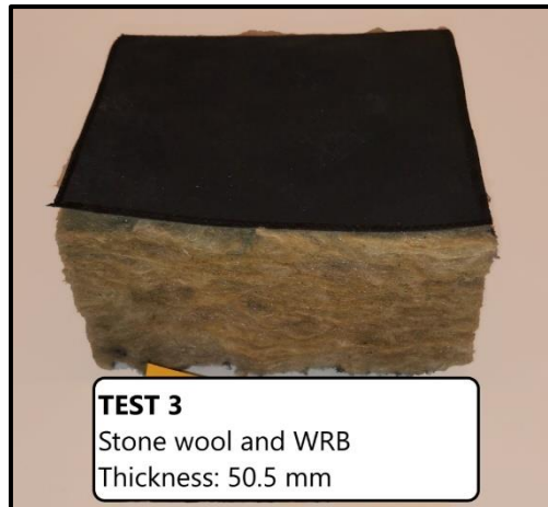
Figure 12: Sample composed of stone wool and WRB
