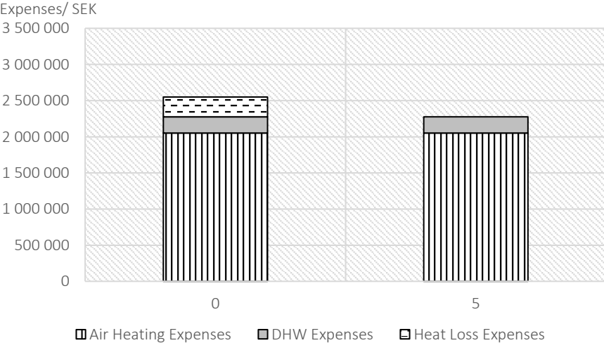
Figure 51 The annual expenses on air and DHW heating energy demand as well as the heat loss through the underground pipes of the Case 0 and Case 5
