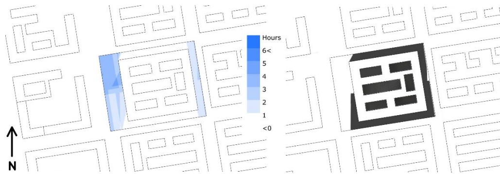
Figure 37 Sun hour condition from 10.00 to 16.00 on 21 st December (left) and the fully shaded area derived from the overlapped shadow domain according to the study in 4.1.2.6 (right).
