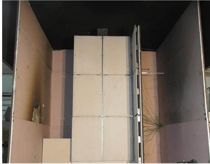
A11. a) Live Fire Test Open Cavity Set-up
