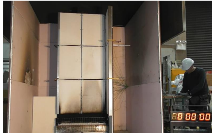
A11. b) Live Fire Test Closed Cavity Set-up
