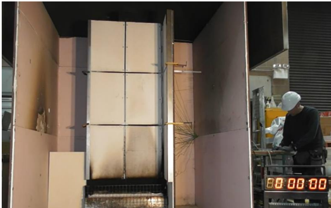
Figure 7: Experimental Configuration for the 50mm Closed Lateral Ventilation Façade sample
