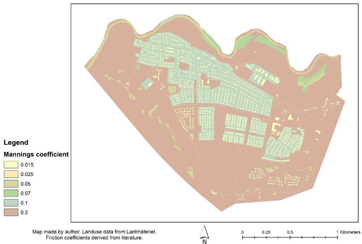
Figure 6: A map showing the friction values used for input to the model.
