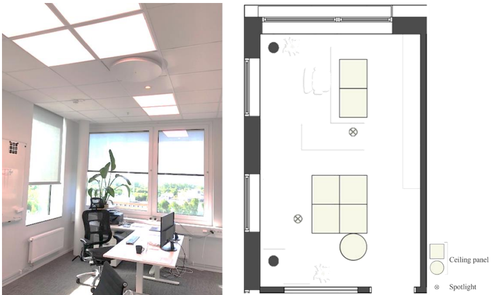
Figure 10: Luminaires distribution in one of the selected offices
