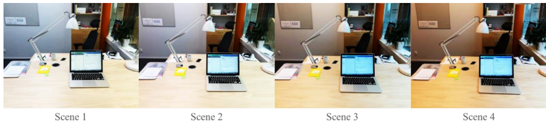
Figure 8: The light starts with a bright blue light in the morning with Scene 1 and gradually dims down towards a warmer red light in the afternoon with Scene 4
